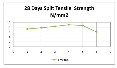
As shown in the graph: 28 days strength is analyzed at 0%, 1%, 2%, 3%, 4% and 5% replacement by bacteria, and split tensile strength is increased by 6.72%, 14.54%, 23.87% and 19.48% respectively as compared to the conventional concrete mix and decrease 17% when 5% bacteria mixed.
