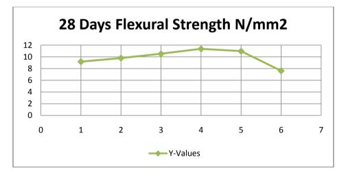
As shown in the graph: 28 days strength is analyzed at 0%, 1%, 2%, 3%, 4% and 5 replacement by bacteria, and flexural strength is increased by 6.74%, 14.58%, 23.83% and 19.97 respectively as compared to the conventional concrete mix and decrease 16.71% when 5% bacteria mixed.
