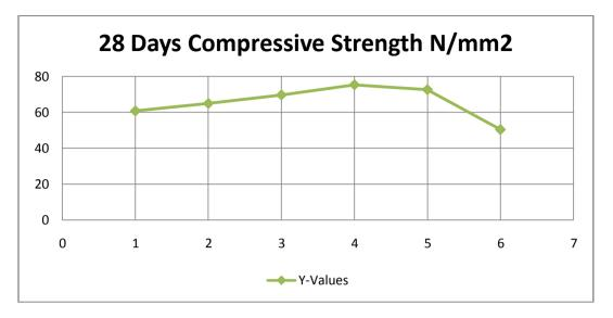
As shown in the graph: 28 days strength is analyzed at 0%, 1%, 2%, 3%, 4% and 5% replacement by bacteria, and compressive strength is increased by 7.15%, 15%, 24.36% and 19.9 respectively as compared to the conventional concrete mix and decrease 16.71% when 5% bacteria mixed.
